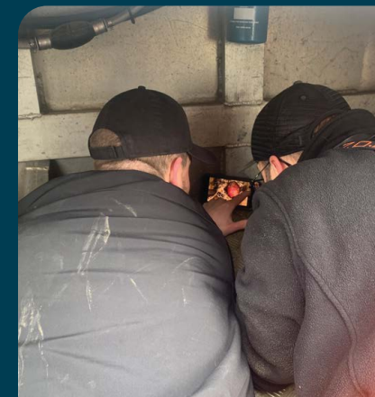
▲ Using an endoscope camera to inspect a boat for aquatic invasive species.
